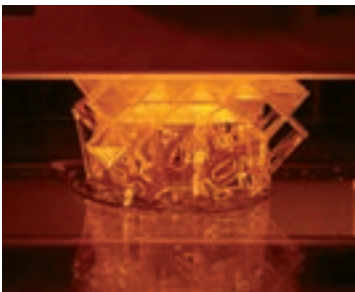
It features proprietary projector lens and Roland's ImagineCure resin, creating 3D models using UV light.
