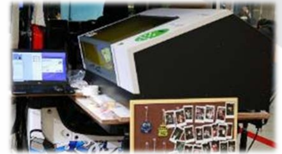
Designs created by visitors were printed directly onto key chains using the LEF-12i UV printer
